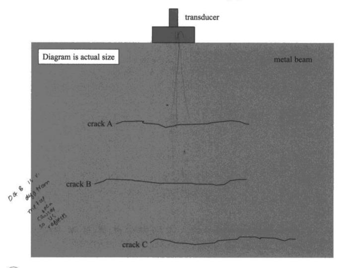
The transducer detects a returning pulse from each crack.
