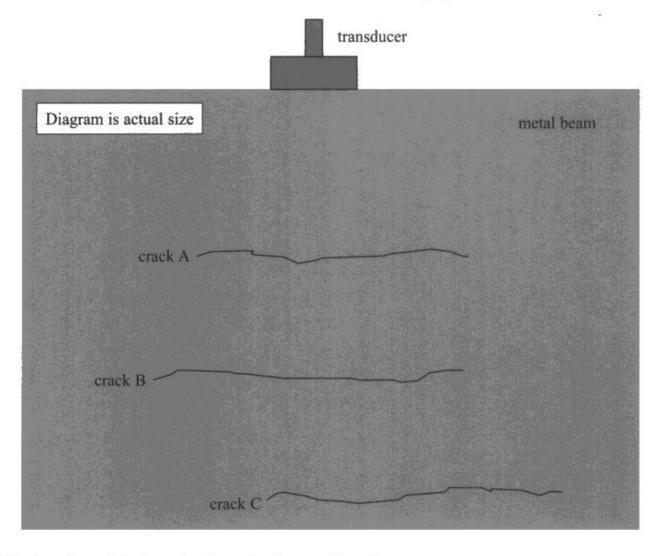
The transducer detects a returning pulse from each crack.
