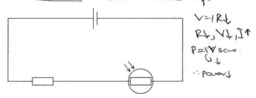
Explain why the power dissipated by the whole circuit changes as the intensity of the light incident on the LDR increases.
