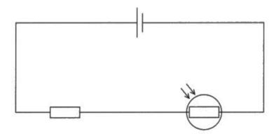
Explain why the power dissipated by the whole circuit changes as the intensity of the light incident on the LDR increases.
